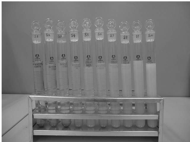
Fig. 1 CePO 4 nanofluids three months after their preparation (reactant molar concentration from 0.02 mol/L to 0.2 mol/L).
